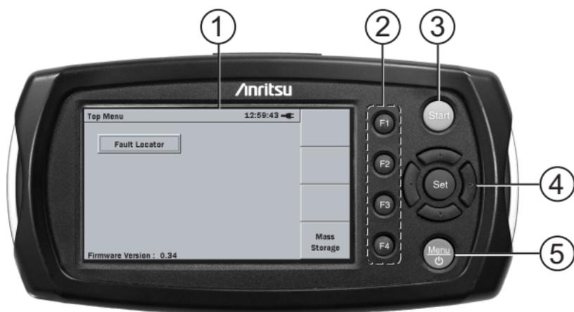
*Figure 2-1: Front Panel layout*
