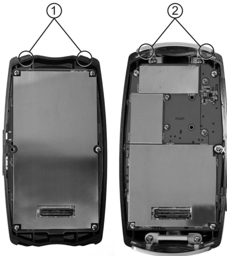
*Figure 2-12: Alignment Tabs and Slots*
