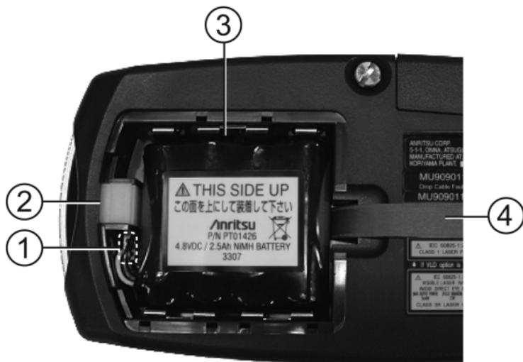
Figure 2-3: Battery Compartment – opened
